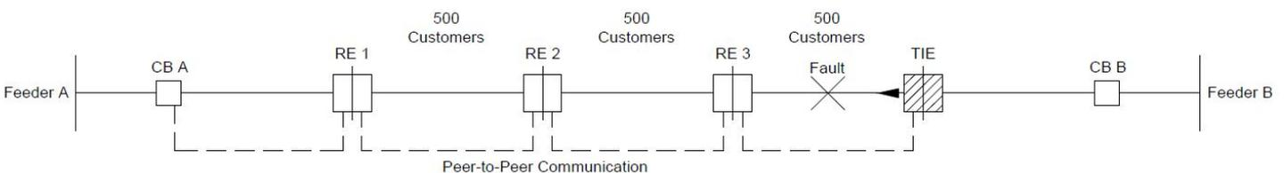
Fig. 5. DA scheme with peer-to-peer communication
