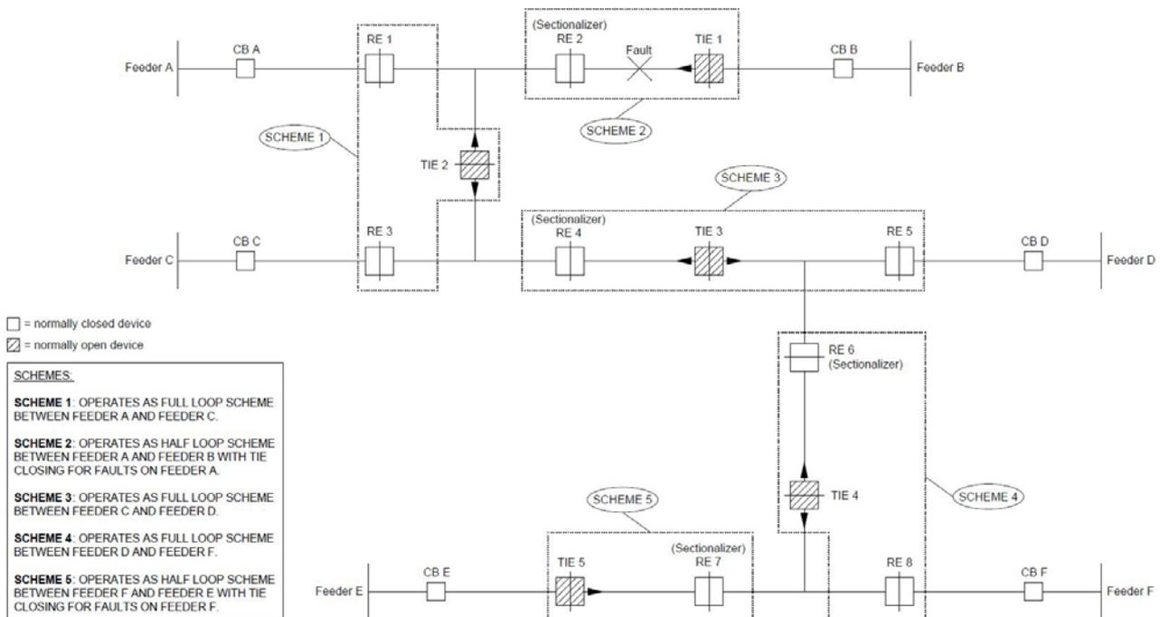
Fig. 4. Complex Loop Scheme Example
