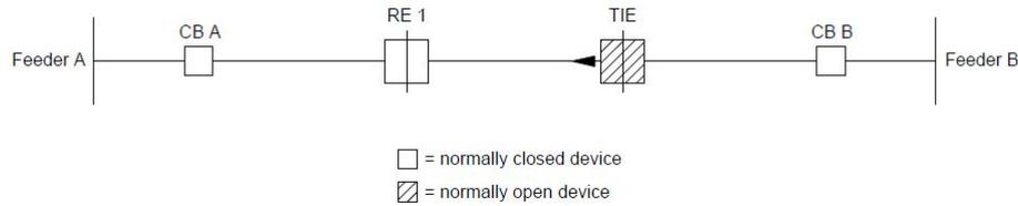
Fig. 1. Half LS with no peer-to-peer communication
