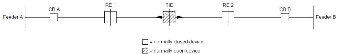
Fig. 2. Full LS with no peer-to-peer communication
